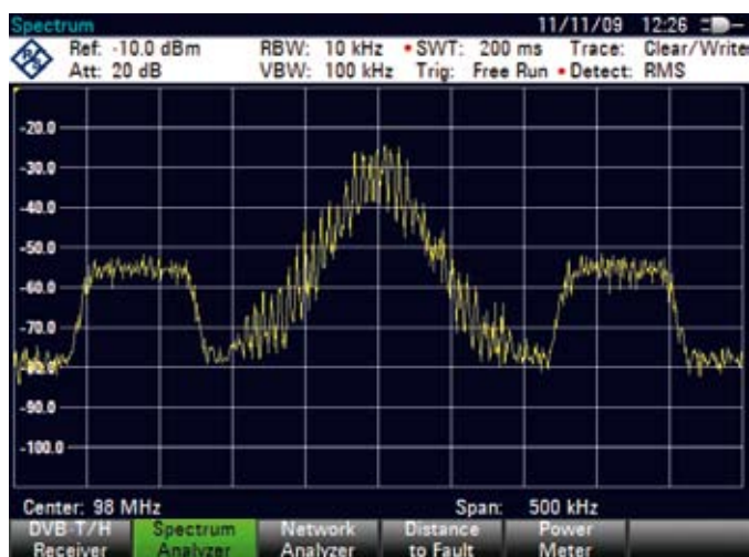
Signal generation for HD Radio™ with the R&S®SFE100-K35 ARB waveform generator.
